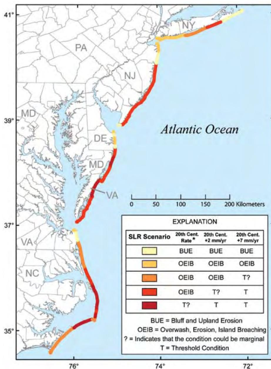
**Figure ES.1** Potential mid-Atlantic coastal landform responses to three sea-level rise scenarios (in millimeters [mm] per year [yr]). Most coastal areas are currently experiencing erosion, which is expected to increase with future sea-level rise. In addition to undergoing erosion, coastal segments denoted with a “T” may also cross a threshold where rapid barrier island migration or segmentation will occur.
