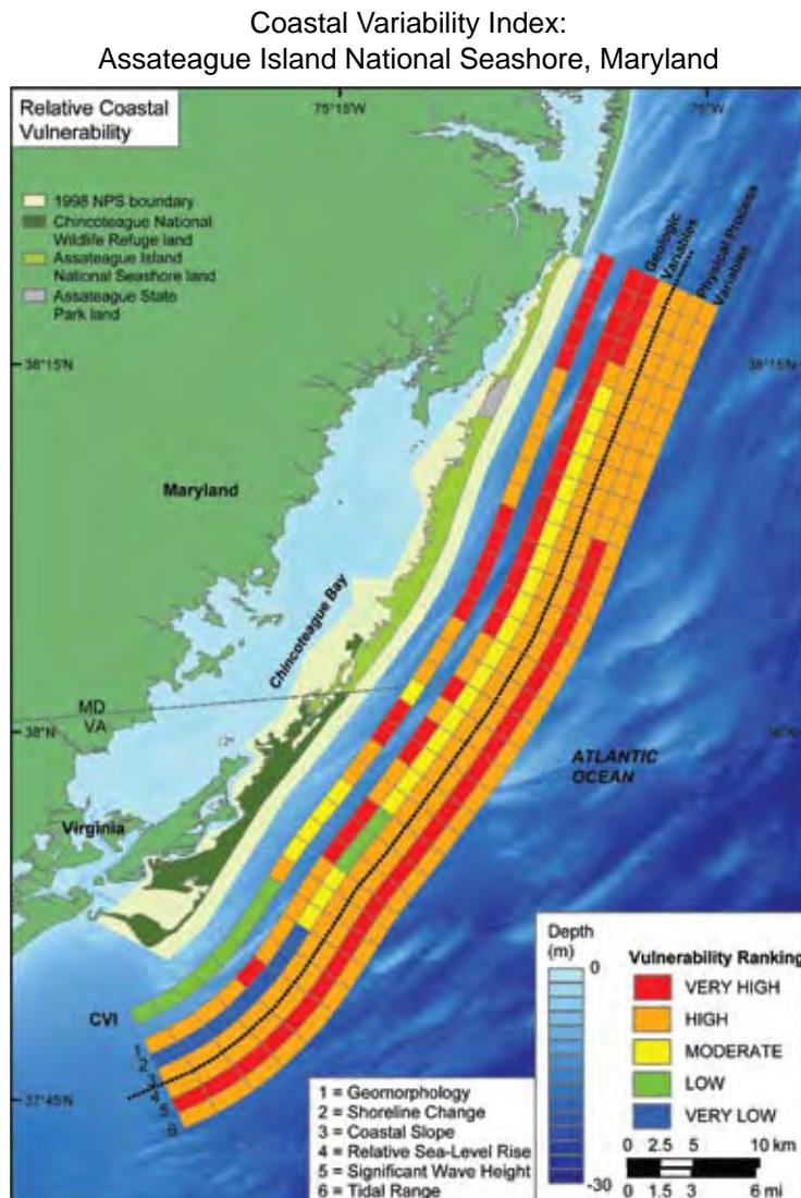
**Figure A2.4** Coastal Vulnerability Index (CVI) calculated for Assateague Island National Seashore in Maryland. The inner most color-coded bar is the CVI estimate based on the other input factors (1 through 6). From Pendleton et al. (2004).
