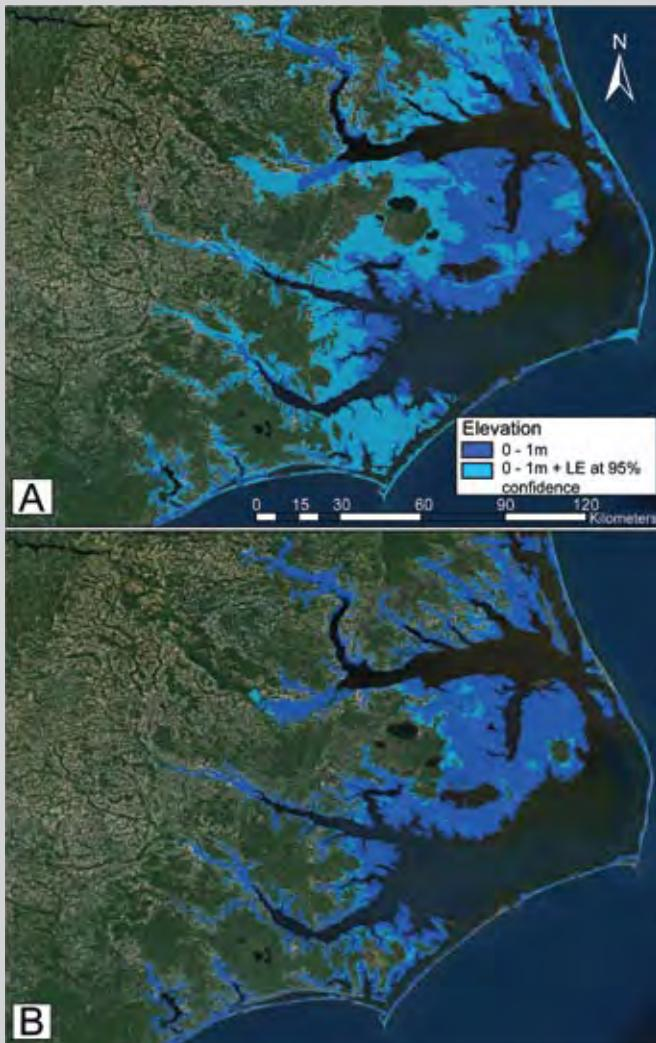
**Box Figure 2.1** (A) Lands vulnerable to a 1-meter sea-level rise, developed from topographic map-derived DEMs and (B) lidar elevation data (Gesch, 2009). The background is a recent true color orthoimage.
