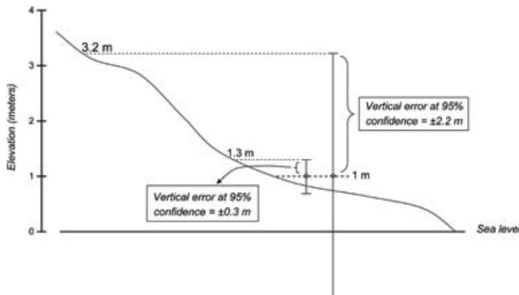
**Figure 2.2** Diagram of how a sea-level rise of 1 meter is mapped onto the land surface using two digital elevation models with differing vertical accuracies. The more accurate lidar-derived DEM ( $\pm 0.3$  m at 95-percent confidence) results in a delineation of the inundation zone with much less uncertainty than when the less accurate topographic map-derived DEM ( $\pm 2.2$  m at 95-percent confidence) is used (Gesch, 2009).
