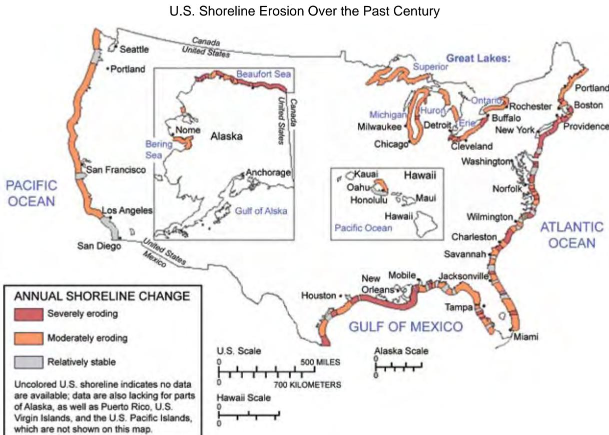
**Figure 1.8** Shoreline change around the United States based on surveys over the past century. All 30 coastal states are experiencing overall erosion at highly variable rates due to natural processes (e.g., storms, sea-level rise) and human activity (From USGS, 1985).
