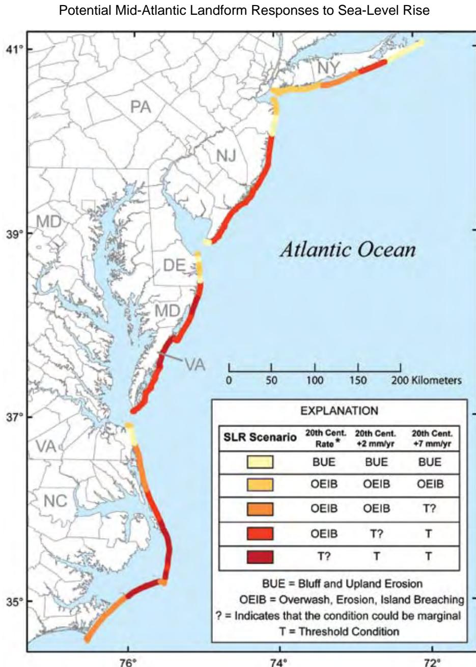
**Figure 3.2** Map showing the potential sea-level rise responses (in millimeters [mm] per year [yr]) for each coastal compartment. Colored portions of the coastline indicate the potential response for a given sea-level rise scenario according to the inset table. The color scheme was created using ColorBrewer by Cindy Brewer and Mark Harrower. After Gutierrez et. al. (2007).
